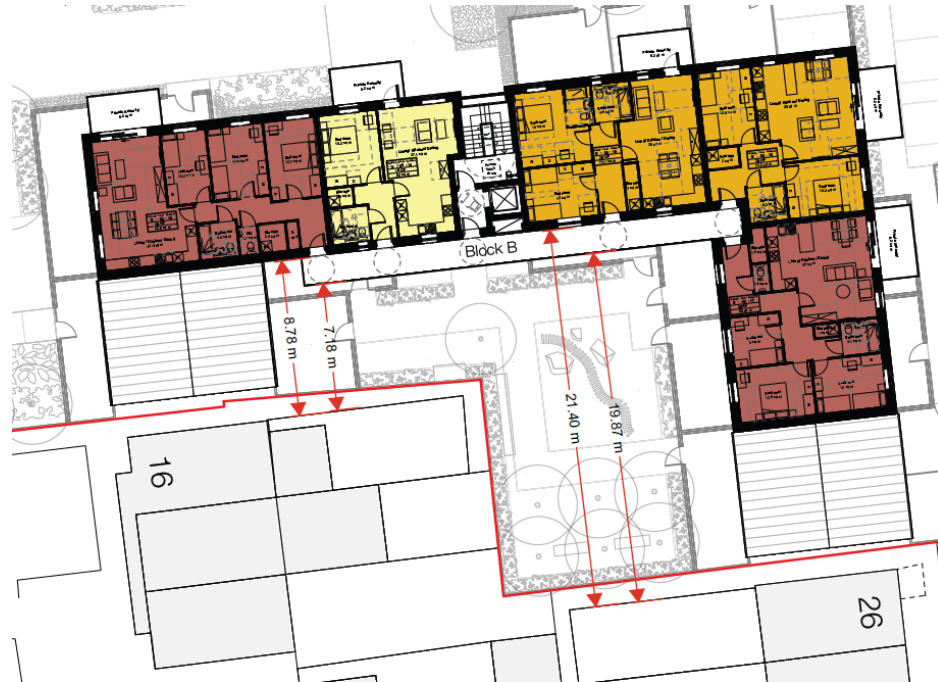
Figure 7: Block B distance between neighbouring properties.
