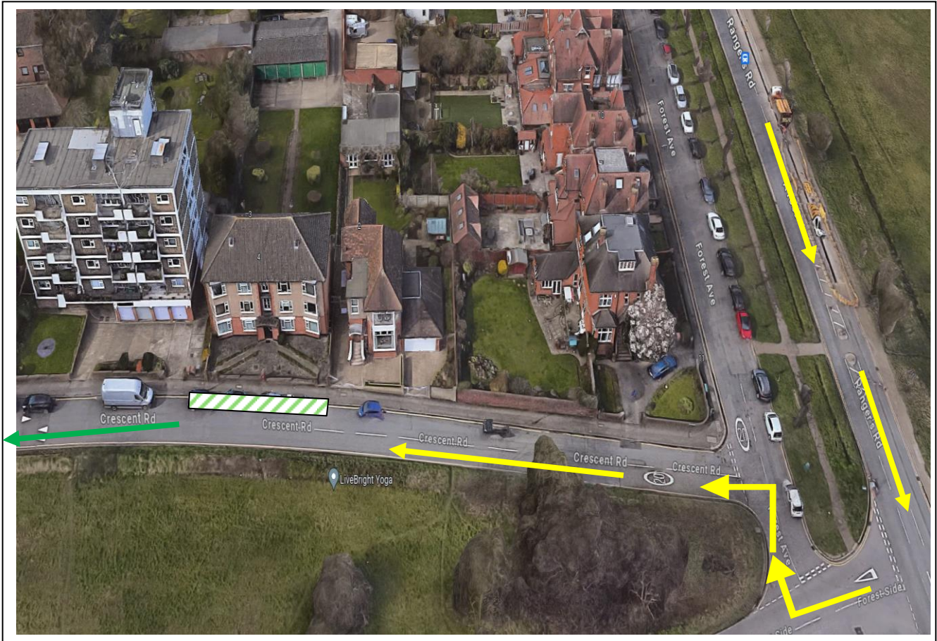
Figure 5: Site layout showing the proposed unloading arrangements.
