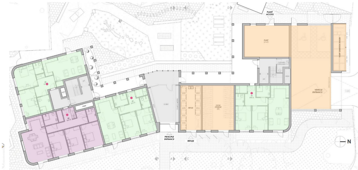
Figure 4: Ground floor plan, showing the entrance lobby, rear yard area and location of dual building cores.
