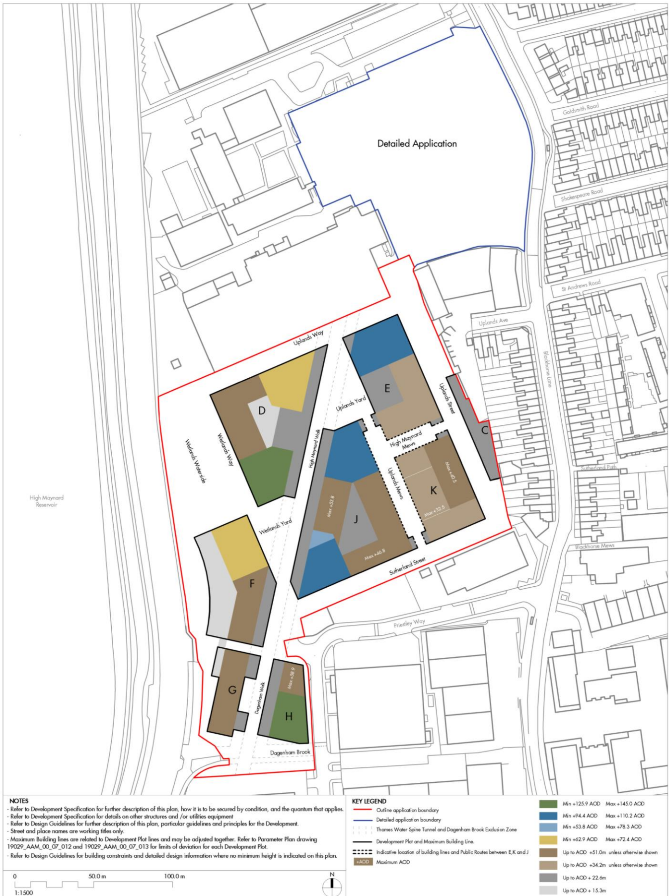
Figure 7: Minimum and maximum building heights – Phase 2
