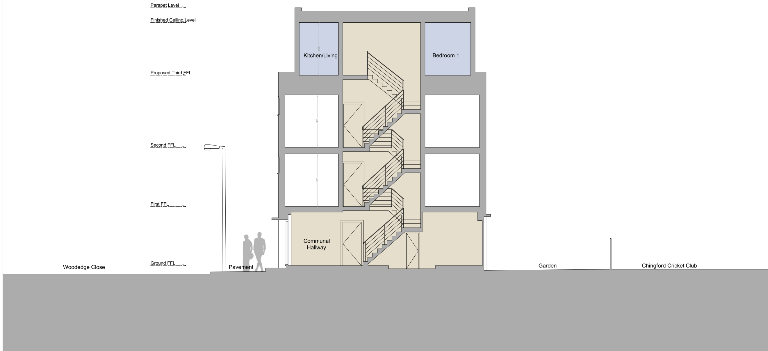
Proposed Section A-A (1:100 @ A3)
