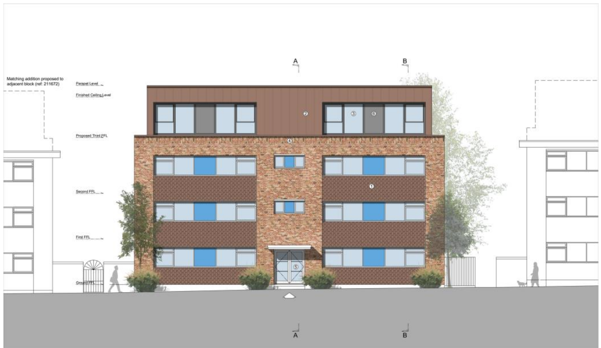
Proposed Front Elevation (1:100 @ A3)
