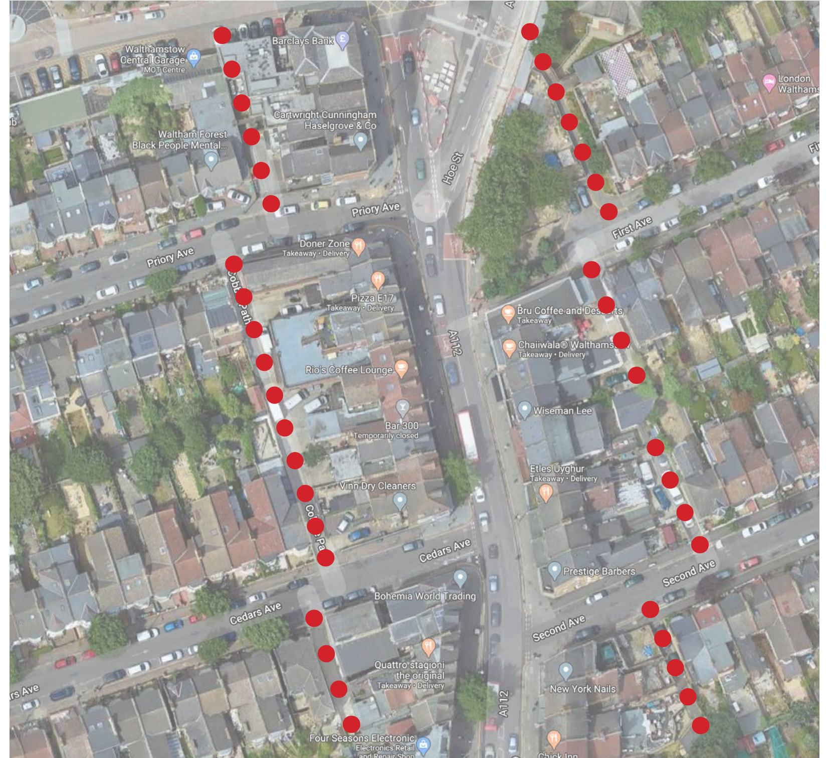
Diagram Showing Secondary Service Routes Running Parallel To Hoe Street
