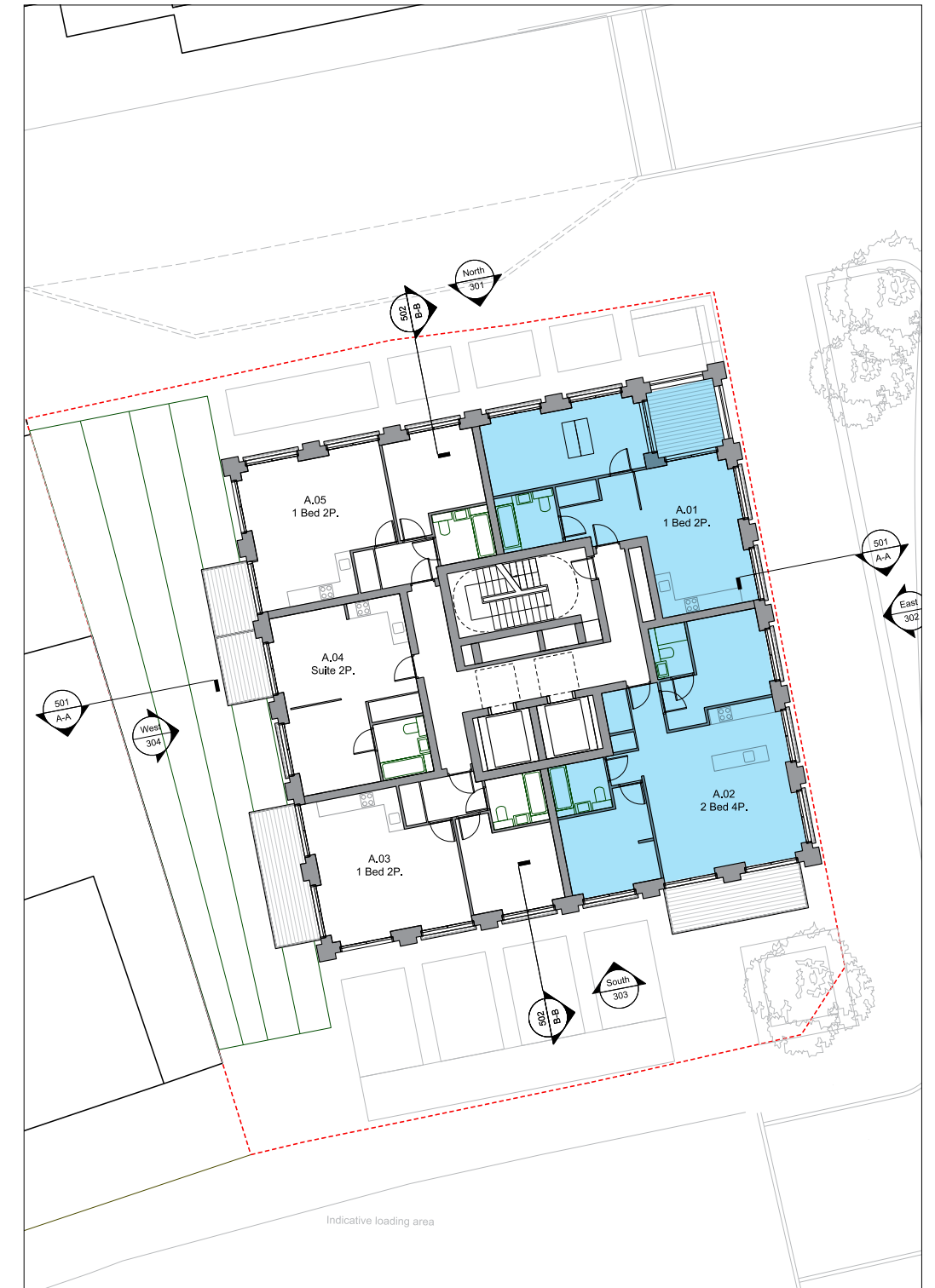
2nd Floor Plan Showing Location of Wheelchair Apartment Types
