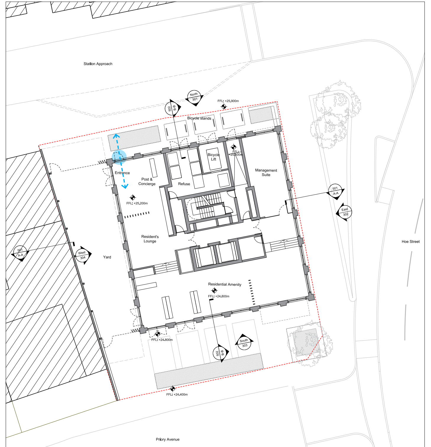
Ground Floor Plan Showing Emergency Door
