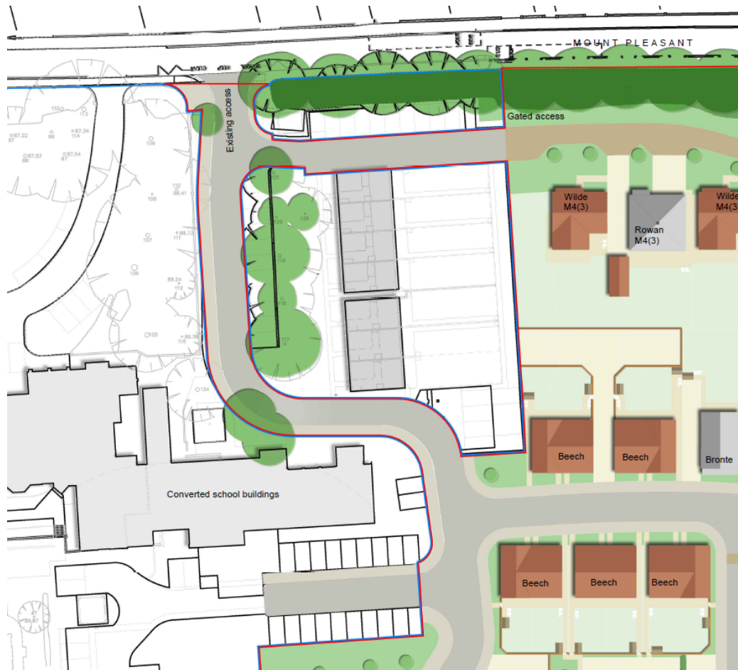
Figure 6 – Extract from the Proposed Site Layout (Coloured) Plan (23110 (D) 005) which demonstrates the main vehicular access into the site
