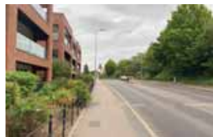
Figure 5.14. Examples of zebra crossing with adequate visibility (top) and a clear 2m wide footway (Radvinter Road, bottom)
