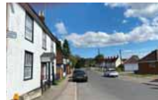
Figure 6.14. Example of footway parking compromising effective footway width
