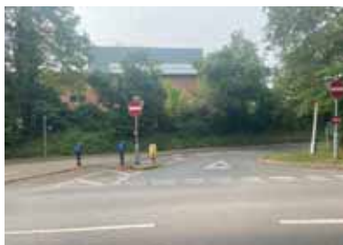
Figure 5.9 Example of contraflow access for cyclists on one-way street improves directness (Wenden Road)
