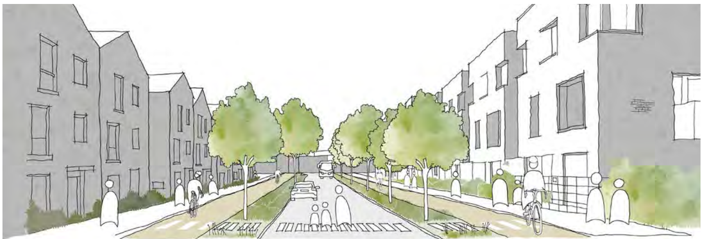
▲ Above is an illustrative sketch for a successful Market Street. It contains key features such as wide footways and cycle lanes on both sides of the street, and a range of SuDS and landscaping elements incorporated into the street scene.
