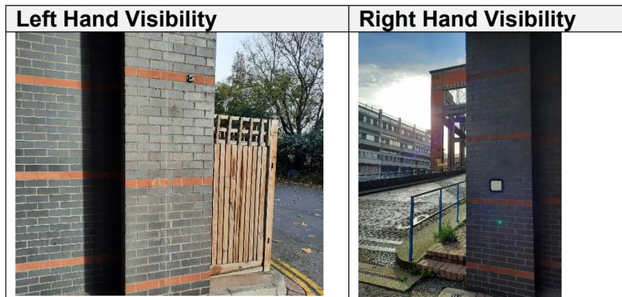
The northern access junction (egress) has been designed as the site egress with a no-entry sign and the building line angled to allow right hand visibility towards vehicles approaching from Observatory Car Park and car parks to the rear of the High Street Shops. A fence appears to have been erected which would need to be removed/reduced to allow suitable visibility.
