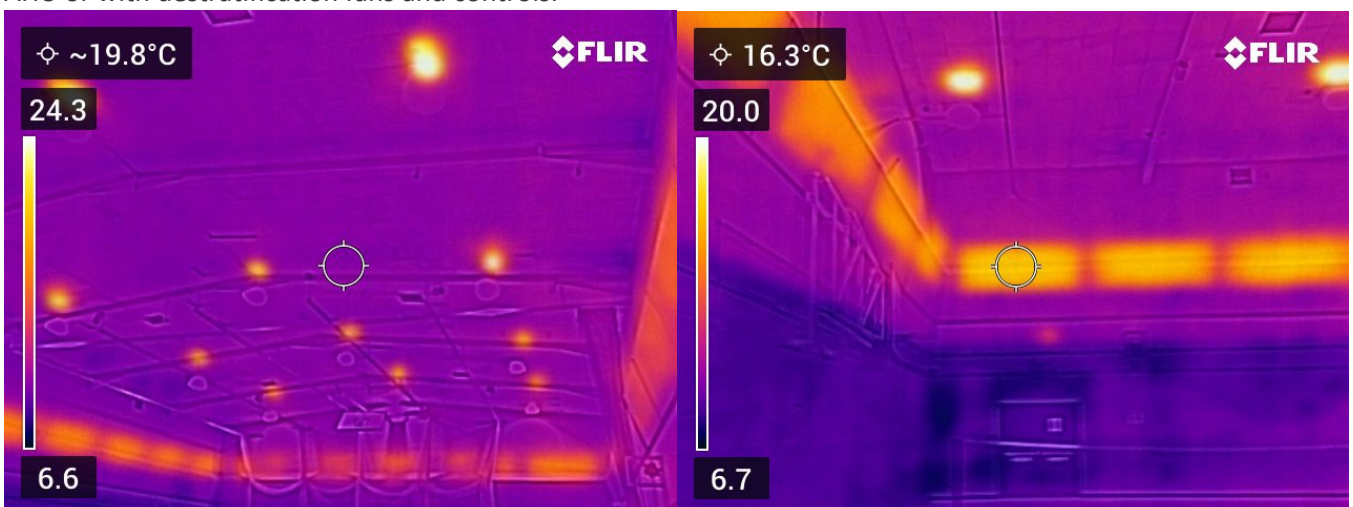
Figure 14: Thermal imaging of heated areas during periods of no use
