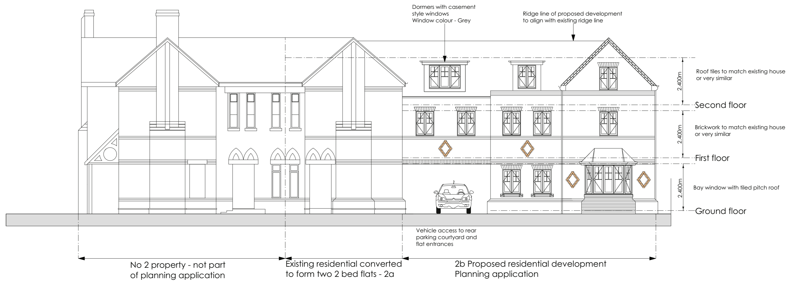
Elevation to Franchise Street Scale 1 : 100
