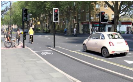
Figure 3.9: Separate cycle signals at junctions
