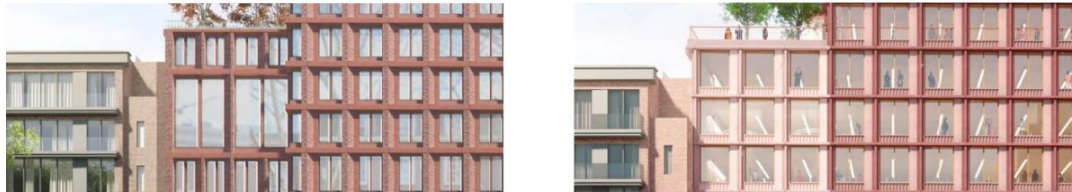
Figure 13: (Left) Original large windows on Grays Inn Road façade: (Right) Revised gridded façade on Gray's Inn Road
