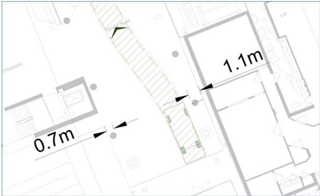
Figure 4. Extract of swept path analysis drawings provided in Appendix B of the Transport Statement.
