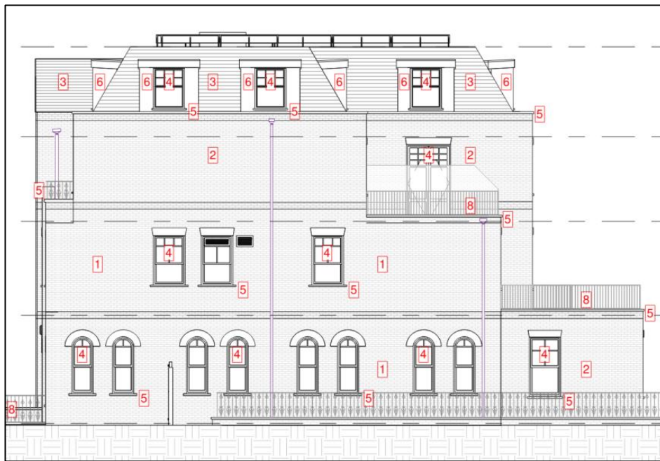
Figure 2 – Proposed 39a FJA side (north) elevation. Windows at ground and first floor are existing, while the roof level windows are new. The rear facing terraces (right) feature privacy screens.
