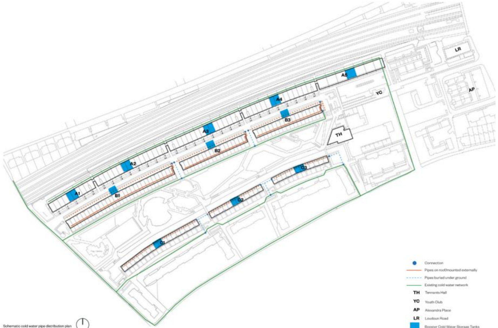
Schematic cold water pipe distribution plan
