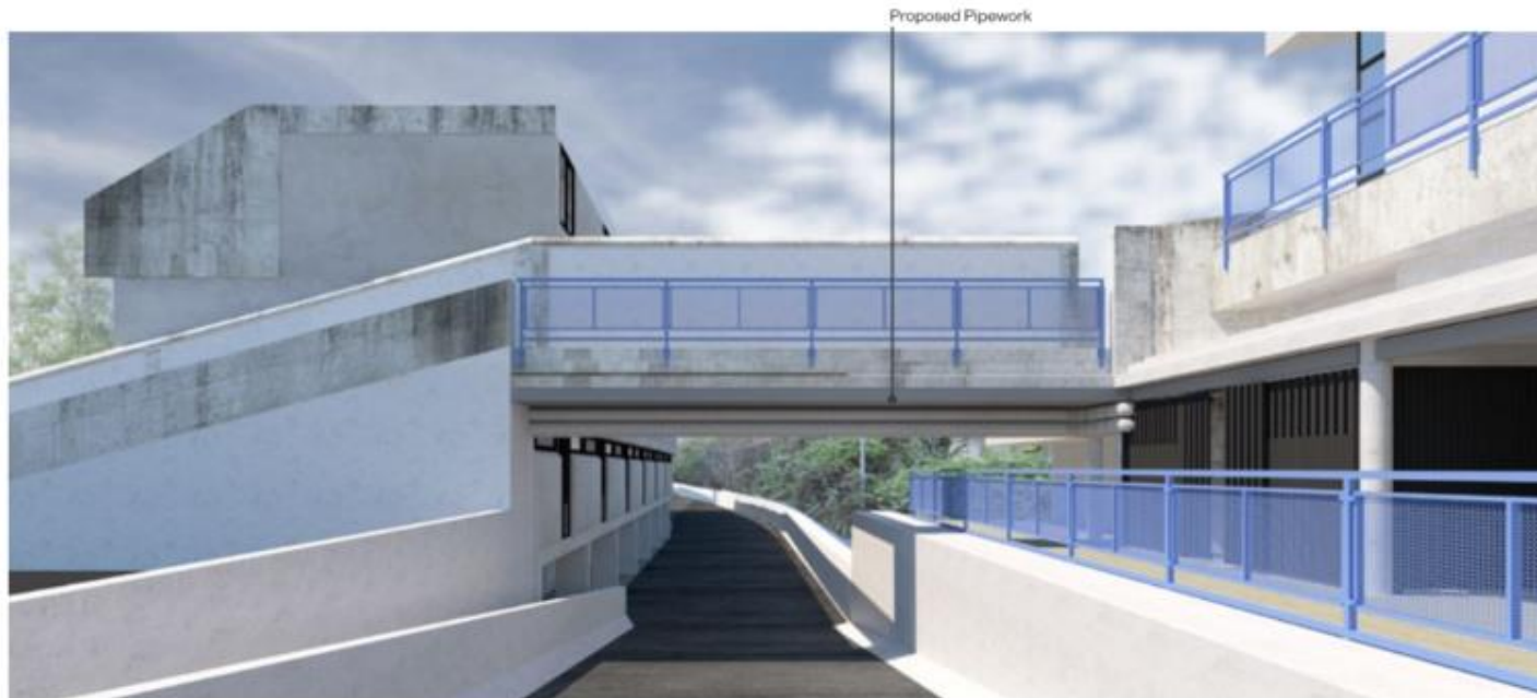
View 1: Bridge link between the community centre & block C seen from east. Proposed pipes fixed to underside of existing bridge
