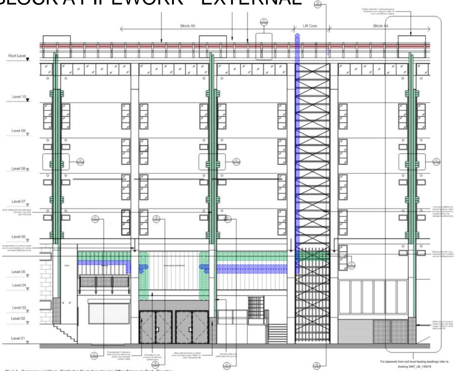
Block A - Temporary and Final - Distribution Route from Housing Office Balcony to Roof - Elevation
