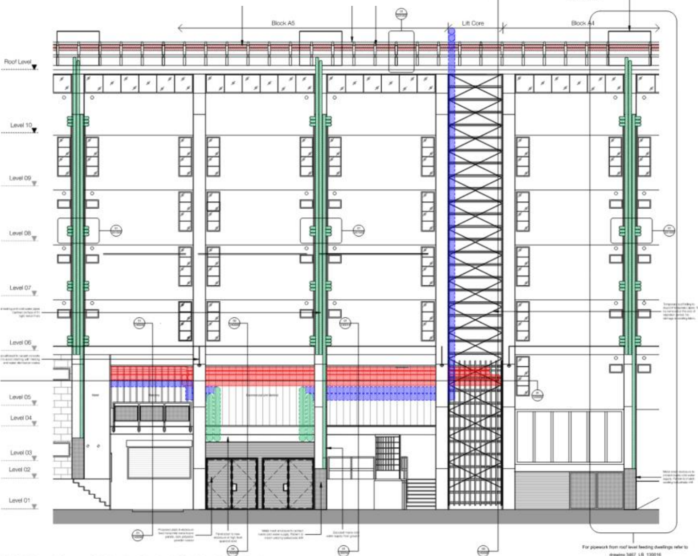
Block A - Existing and Temporary - Distribution Route from Housing Office Balcony to Roof - Elevation 1:50
