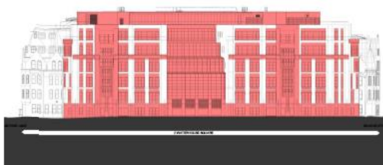
Figure 17. The internal layout and building quality improvements, including new cores, raised floor levels and active ground floor frontages, necessitate the removal of most of the existing granite cladding (areas removed in red).
