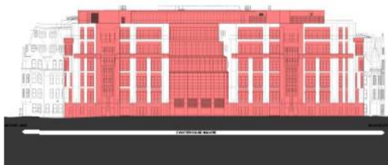
Figure 27. The internal layout and building quality improvements, including new cores, raised floor levels and active ground floor frontages, necessitate the removal of most of the existing granite cladding (areas removed in red).
