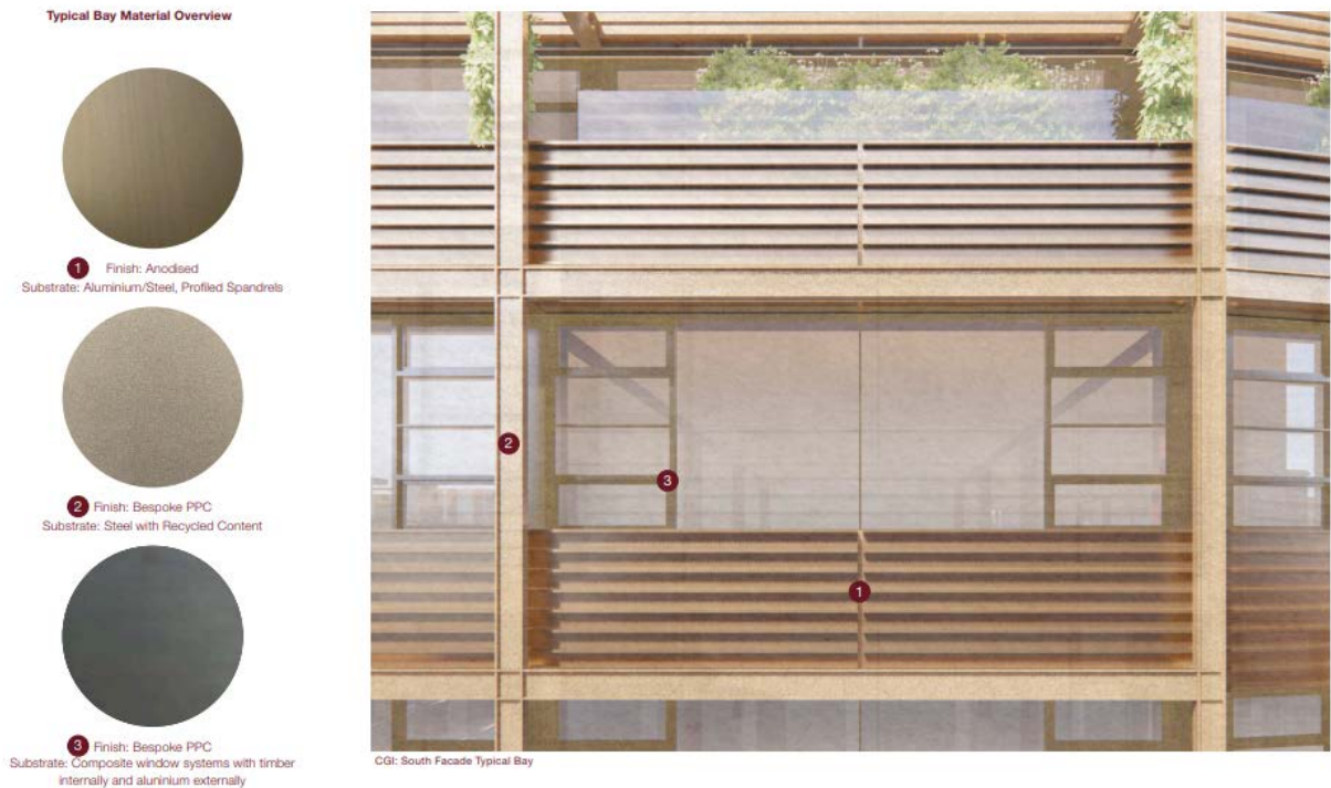
Figure 5: showing typical façade overview and proposed materials
