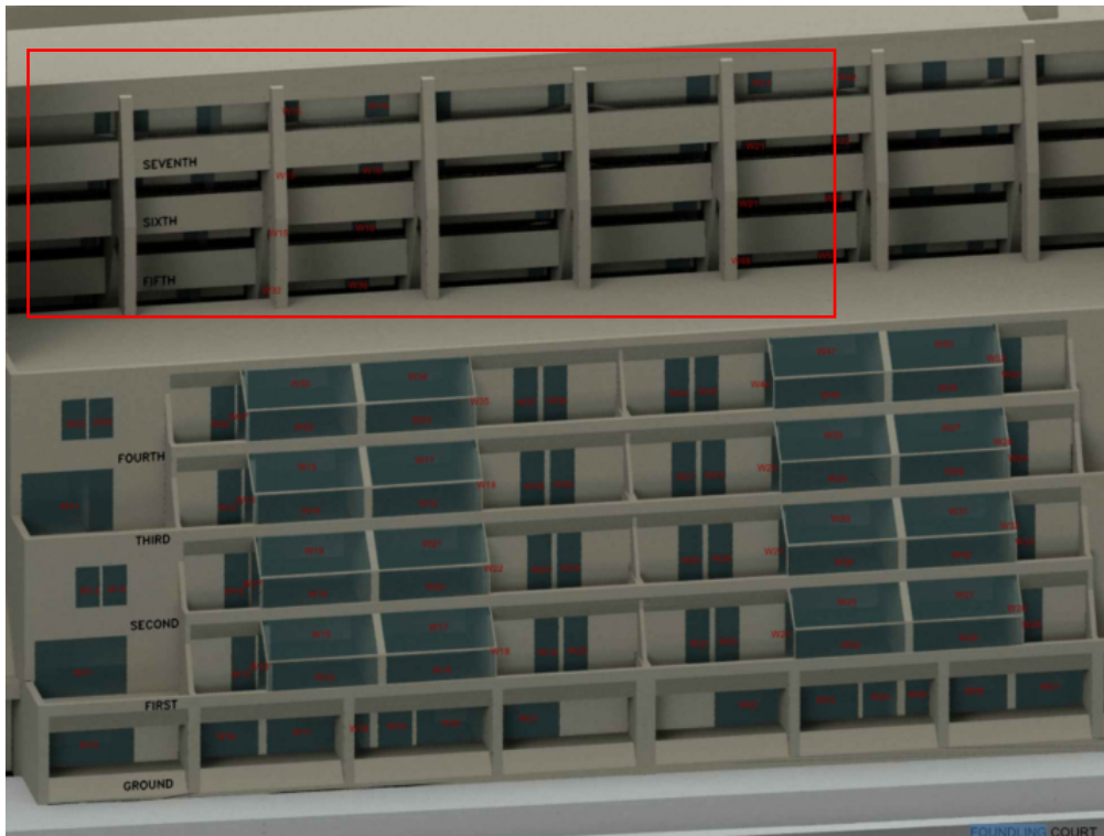
Image 7 – extract from DSL impact assessment showing neighbouring windows that would not meet BRE guidance
