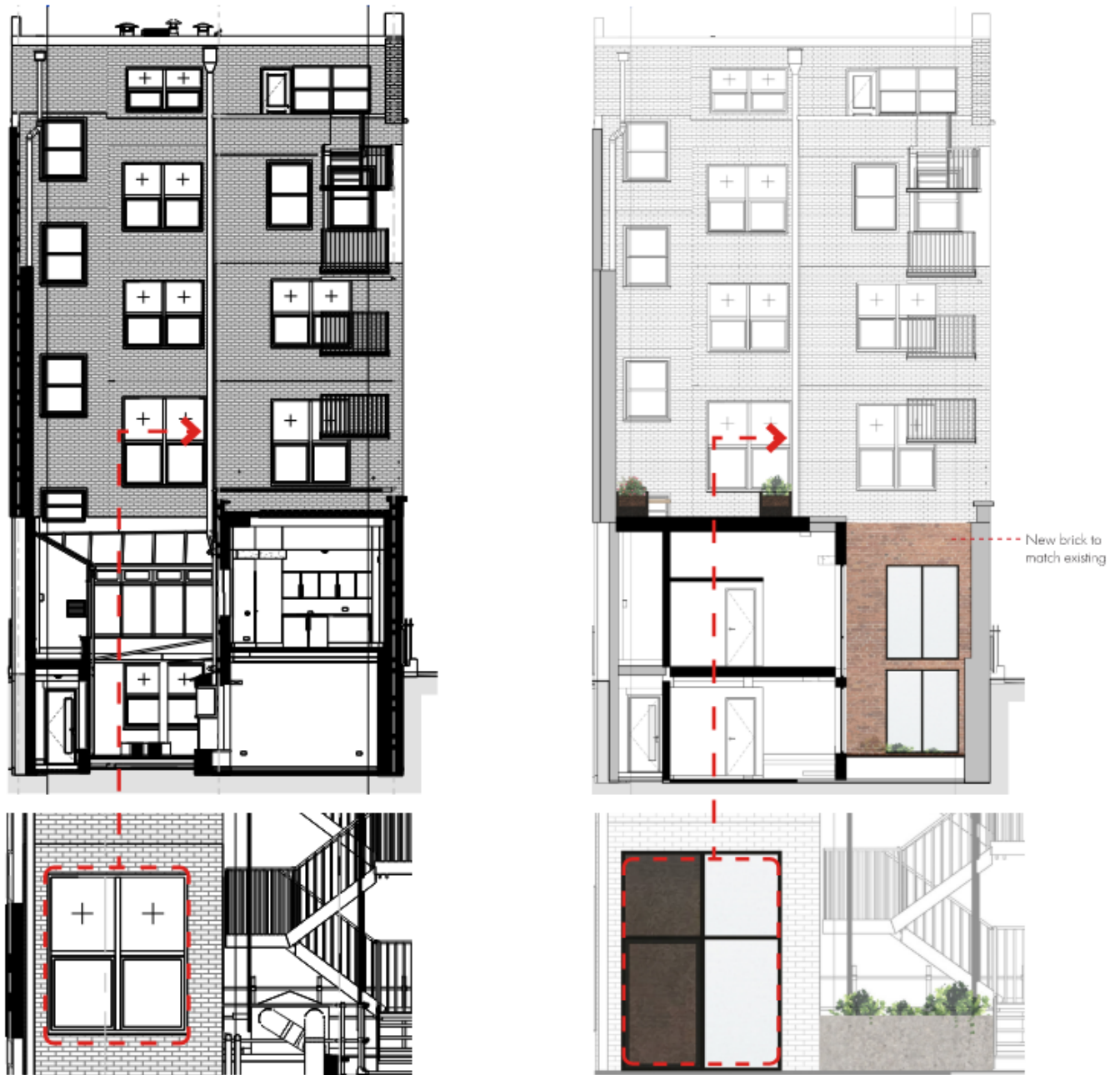
Figure 4 Existing and proposed rear elevation of Bedford Row with link structure partially demolished and replaced
