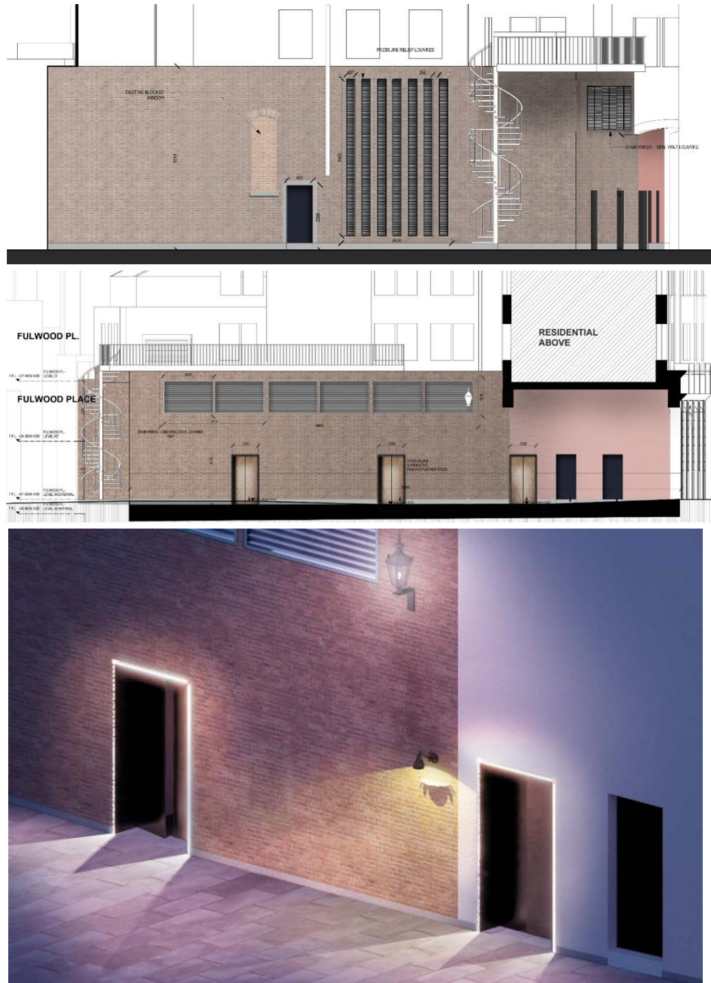
Figure 9: Proposed north (top) and west (middle) elevations and indicative lighting strategy to the passageway (bottom).
