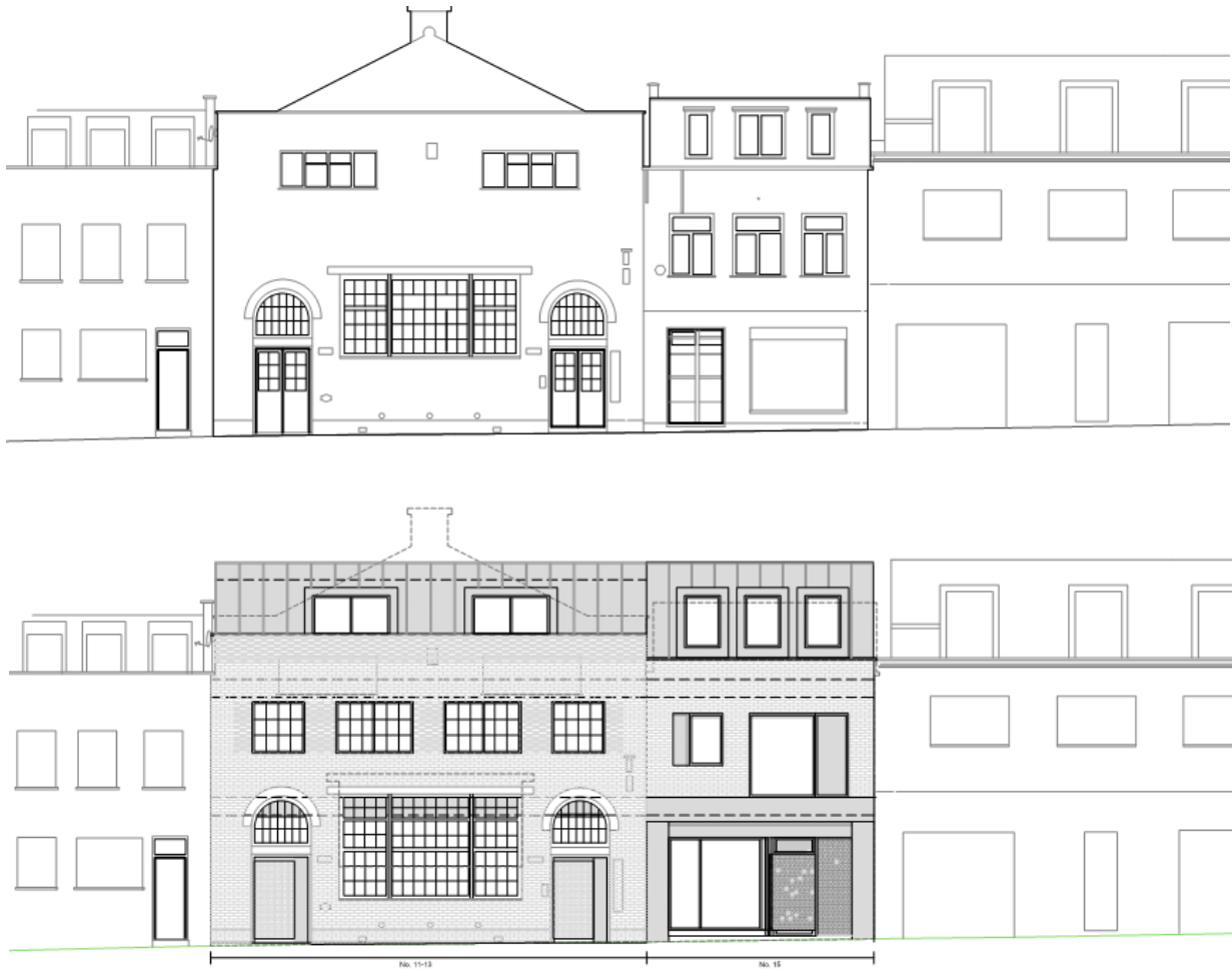
Figure 1: Existing (top) and Proposed (bottom) Street elevation
